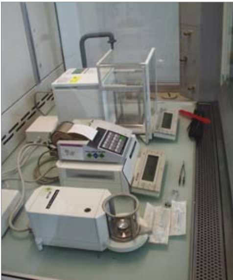
Diag. 37: Workstation WS-AS as protected weighing station with half-micro and micro scales
