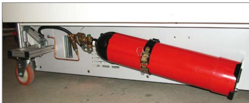
Diag 18: Integrated fire extinguisher
