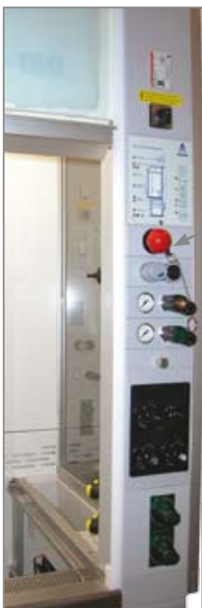
Diag. 17: Security button to release the fire extinguisher
